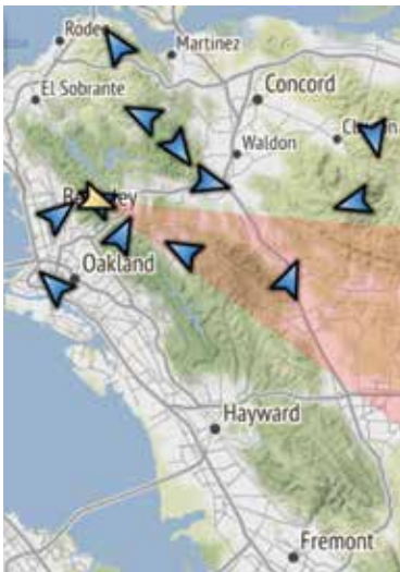
The FUEGO system uses ground-based cameras through networks such as ALERTWildfire. The map above (left) shows locations of cameras in the East Bay. The Vollmer Peak camera (yellow arrow) sees the view above when facing east.
